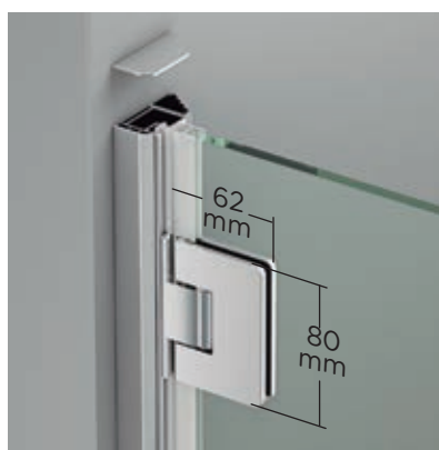
Detalle bisagra cerco-pared Aluminio-Zamak
